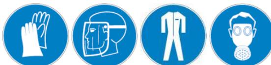
Materials for protective clothing : GIVE GOOD RESISTANCE: natural rubber. nitrile rubber. butyl rubber. polyethylene. PVC. viton. GIVE LESS RESISTANCE: neoprene. polyethylene/ethylenevinylalcohol. GIVE POOR RESISTANCE: leather. PVA. natural fibres.
