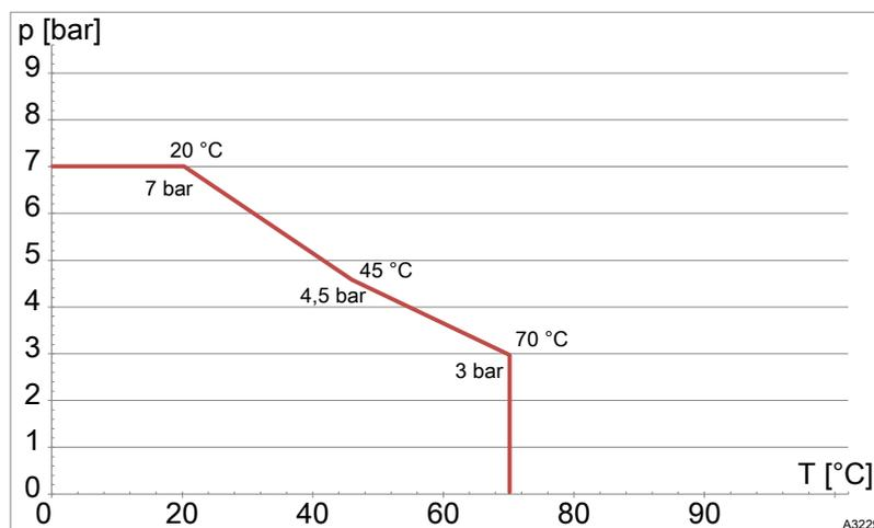
Fig. 21: Pressure / temperature characteristic line, “Industrial water”
