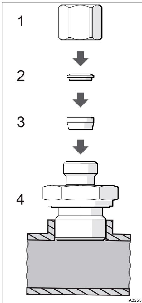
The cutting ring fitting consists of 4 parts:
