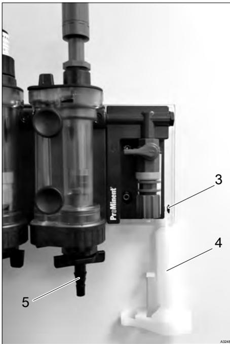
5. ➤ Open the shut-off valve on the inlet side and correctly adjust the flow rate on the ball valve at the outlet side.
