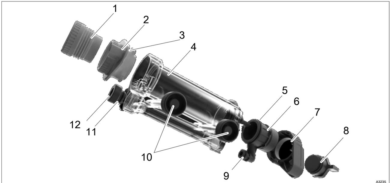
Fig. 18: Construction of the sensor module
