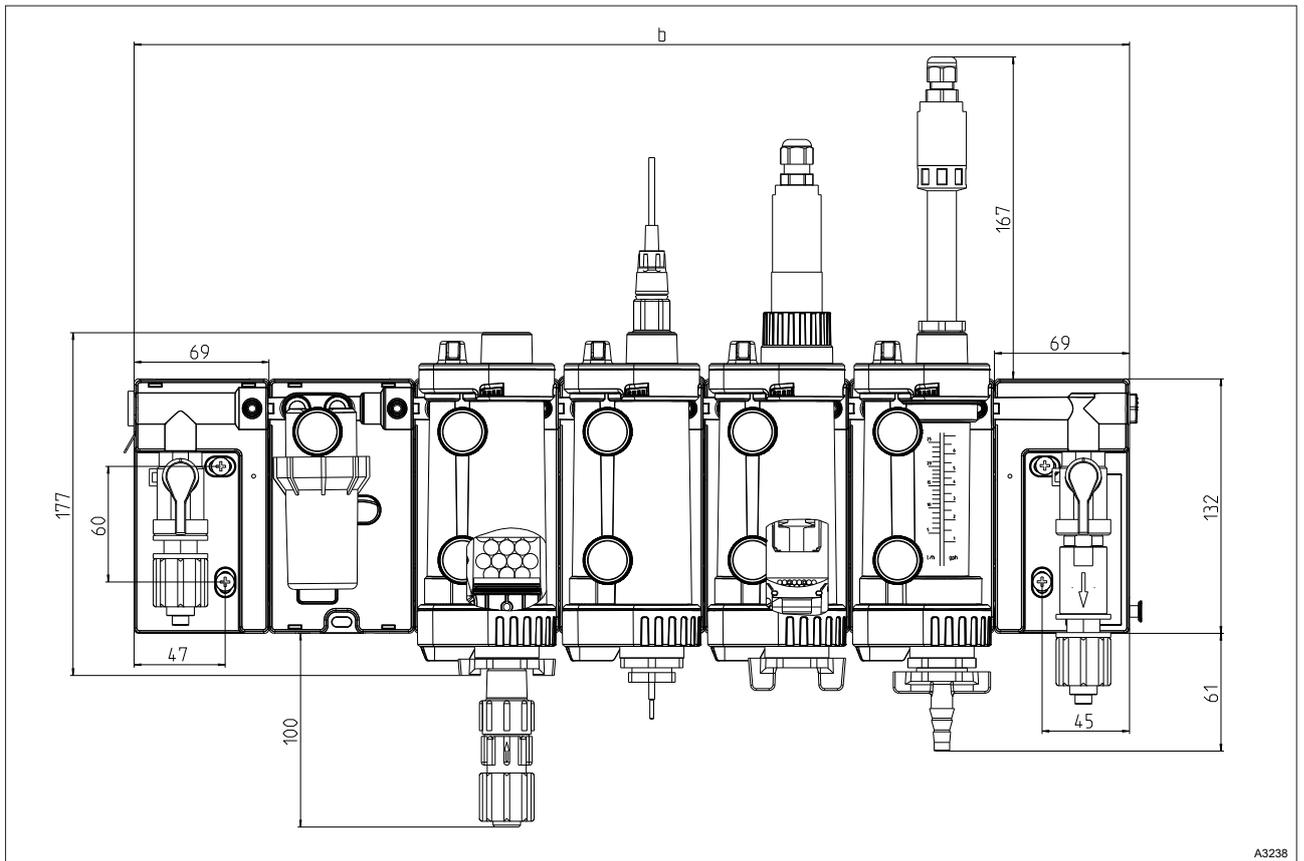
Fig. 23: Example with filter, mixer, pH, CLE and flow sensor
