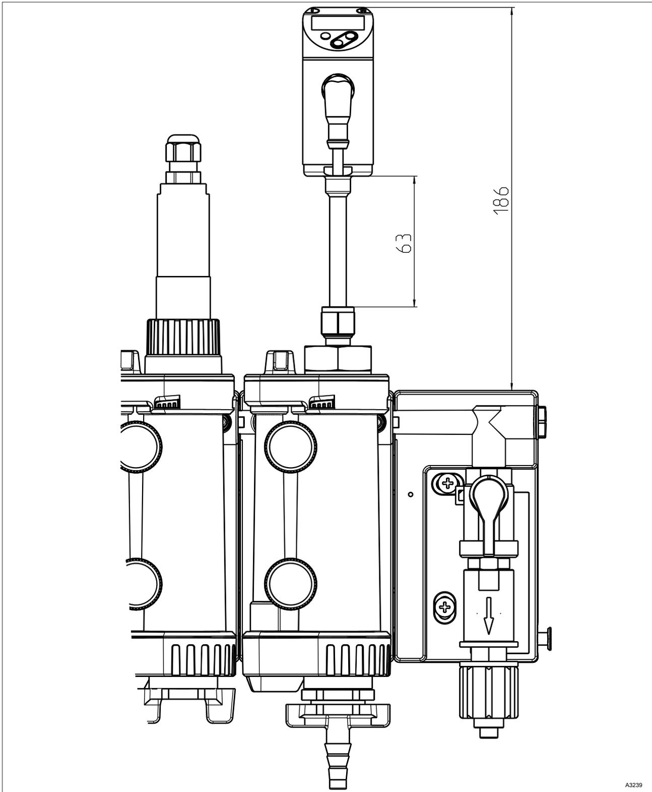
Fig. 22: Bypass fitting with thermal flow sensor
