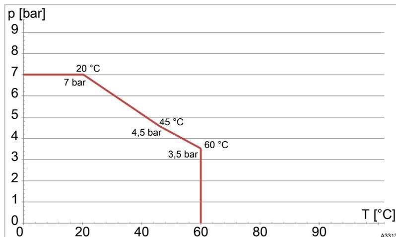
Fig. 20: Pressure / temperature characteristic curve, “Drinking water” / “Pool + Wellness”
