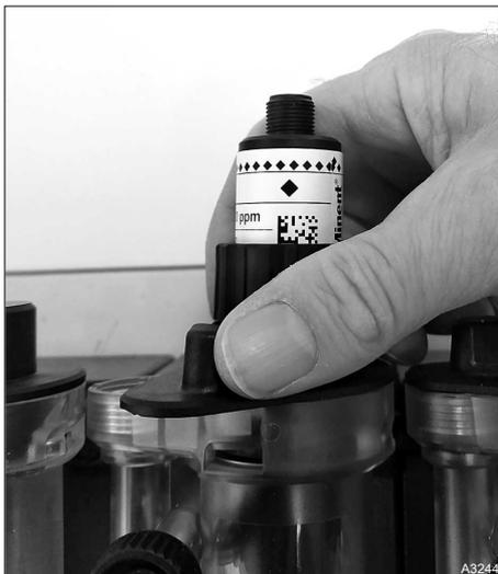
Fig. 12: Assembling the sensor in the sensor module
