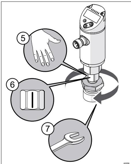
Fig. 9: Tightening the union nut
