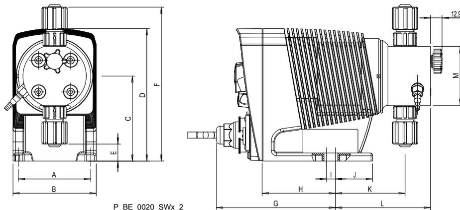
Fig. 20: Dimensional drawing Beta b BT4b/BT5b, material version NP - dimensions in mm
