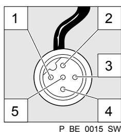
Fig. 10: Cable assignment
