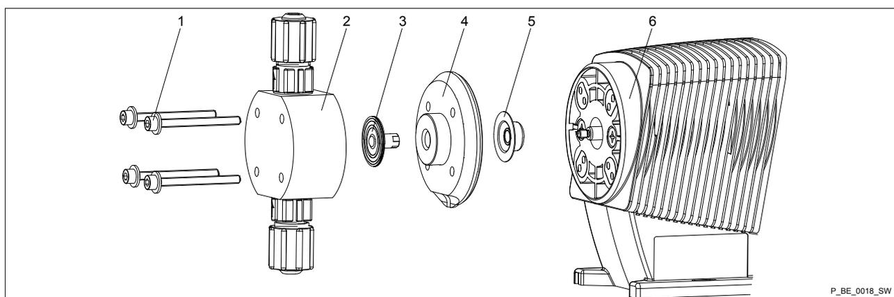
Fig. 18: Partially exploded view of the liquid end
