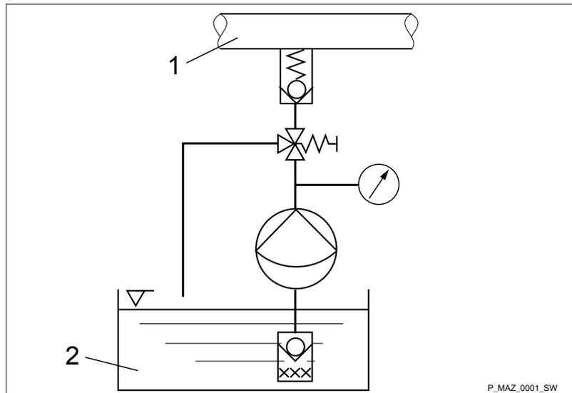
Fig. 8: Standard installation
