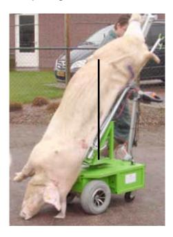
Preferably the guide should walk in front of the machine so that he has better visibility of the route to be followed. Use a thick bag to prevent leakage.
