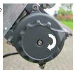
Turning the winch to the freewheel position
