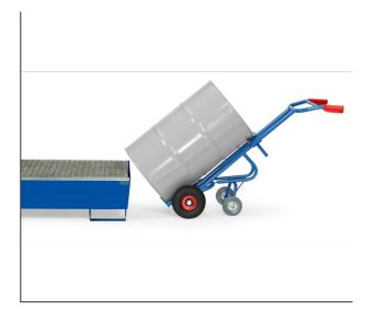
Welded tubular steel, powder-coated, RAL blue 5007, durable surface protection. Wheels with pneumatic tyres, hubs with roller bearings. Suitable for all rimmed 200 litre drums. With 2 additional supporting castor wheels made of solid rubber. With this version, filled barrels can easily be loaded and unloaded from pallets.
