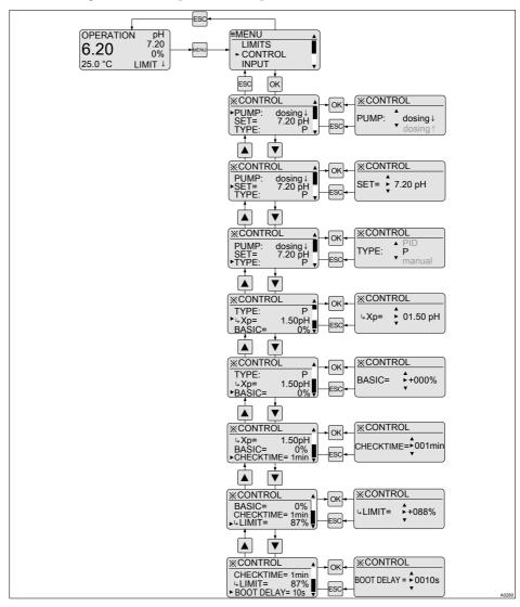
Fig. 29: Setting the control [CONTROL]
