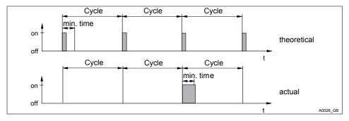
Fig. 37: Theoretical switching time < min. time
