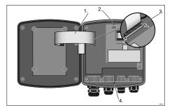
Fig. 47: Fix the ribbon cable
