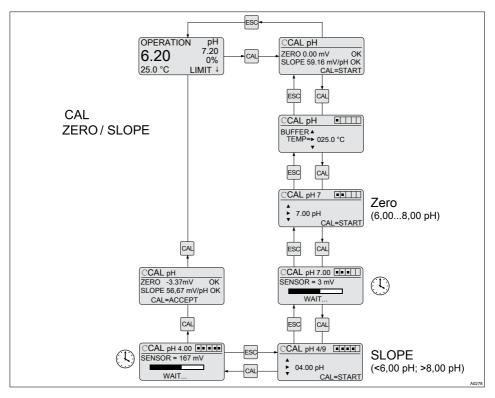
Fig. 24: 2-Point calibration pH sensor
