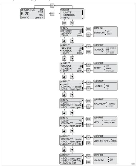
Fig. 30: Input setting (INPUT)
