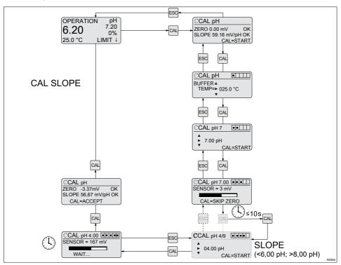
Fig. 25: Single point slope calibration
