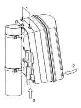
Fig. 6: Suspend and secure the DULCOMETER® Compact Controller
