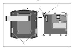
Fig. 51: Removing the strain relief
