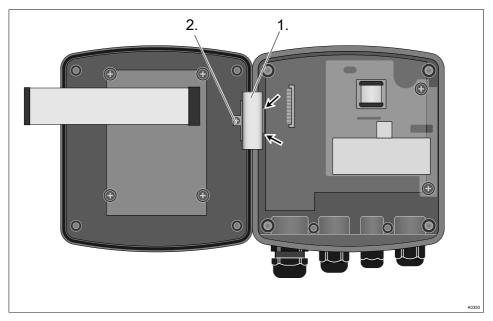
Fig. 9: Dismantle the hinge
