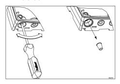
Fig. 16: Punch out threaded holes
