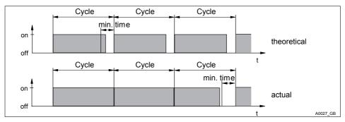
Fig. 38: Theoretical switching time > (cycle - min. time) and calculated switching time < cycle
