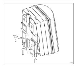
Fig. 5: Removing the wall/pipe bracket
