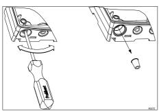
Fig. 46: Punching out the threaded holes
