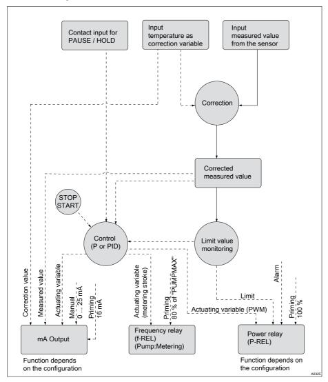
Fig. 1: Flow diagram
