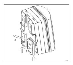
Fig. 3: Removing the wall/pipe bracket
