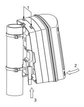
Fig. 48: Suspend and secure the DULCOMETER® Compact Controller
