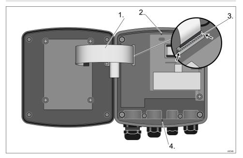
Fig. 8: Loosening the ribbon cable
