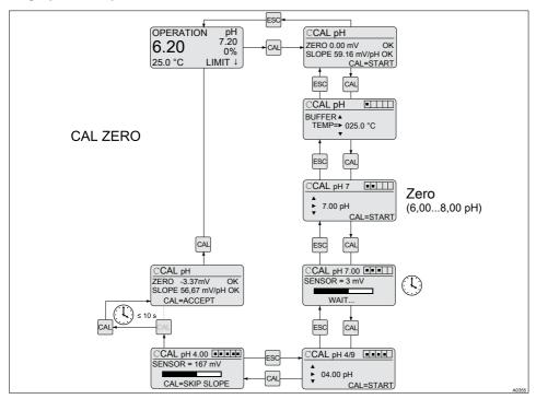
Fig. 26: Single point zero point calibration
