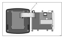
Fig. 42: Pushing and locking the ribbon cable in its base
