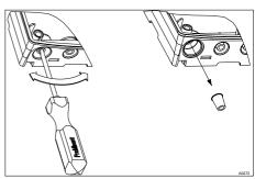
Fig. 52: Punching out the threaded holes
