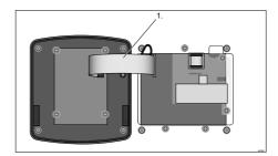
Fig. 49: Loosen the ribbon cable from the base
