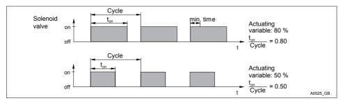
Fig. 36: Solenoid valve (= P-REL: dosing)
