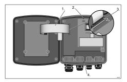
Fig. 39: Loosening the ribbon cable
