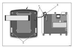
Fig. 54: Fit the profile seal onto the top part of the controller housing
