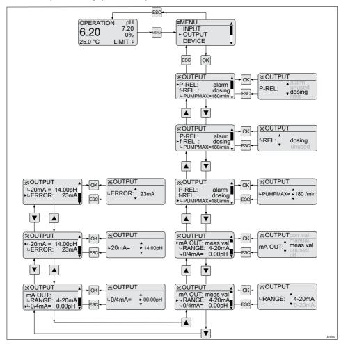
Fig. 31: Output setting (OUTPUT)
