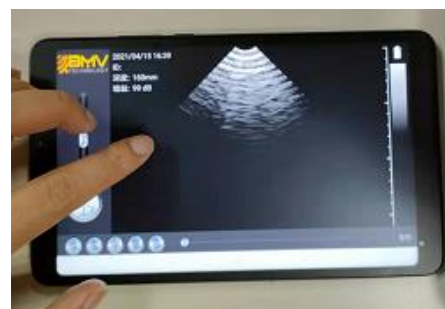
6. Slide up and down in the image area to adjust the depth.
