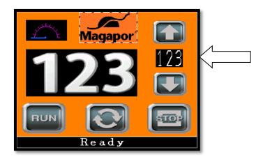
The keys over and below the number button increase and reduce this parameter step by step, which is specially useful for adjusting volume accurately during the run.
