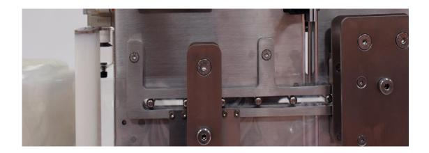
Once verified, press again on the main menu to close the die cutters and move the poles forwards. The equipment is threaded. You can release the blisters now.
