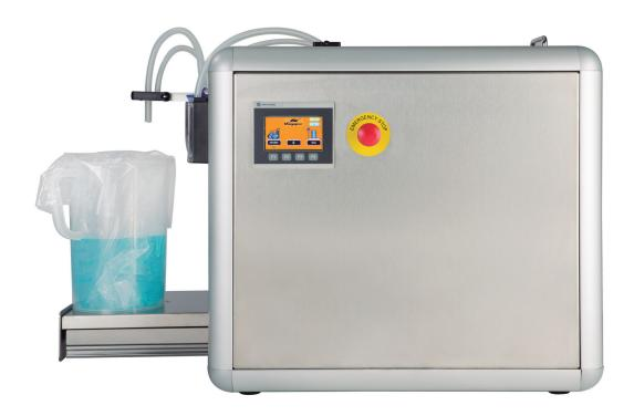
Equipment for preparing reconstituted extender which provides, instantly and at the required temperature, the volume of extender and water necessary for elaborating semen doses.
