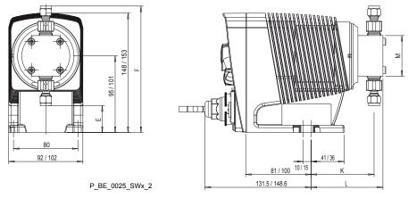
Fig. 25: Dimensional drawing Beta b BT4b/BT5b, material version SS - dimensions in mm
