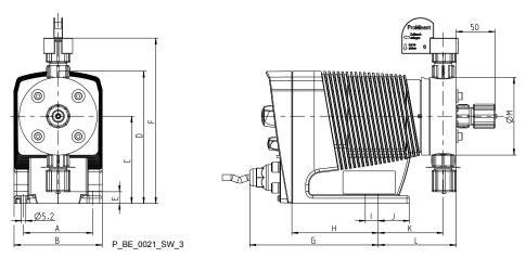
Fig. 21: Dimensional drawing @Beta b BT4b/BT5b, material versions PP and NP with self-bleeding dosing head SEK - dimensions in mm
