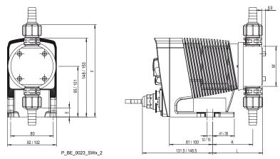
*Fig. 23: Dimensional drawing Beta b BT4b/BT5b, material version PV for high-viscosity feed chemicals - dimensions in mm*
