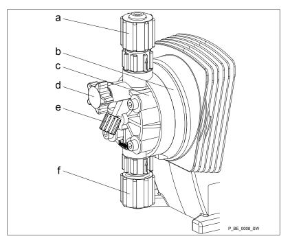
Fig. 3: Overview of liquid end (PV)
