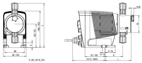
Fig. 19: Dimensional drawing Beta b BT4b/BT5b, material version PP - dimensions in mm
