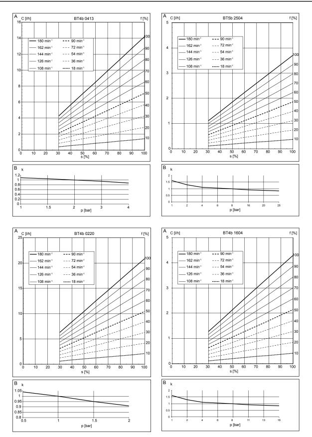
*Fig. 30: A) Capacity C at medium back pressure depending on the stroke length s for different stroke rates f. B) Associated correction factors k depending on the back pressure p.*
