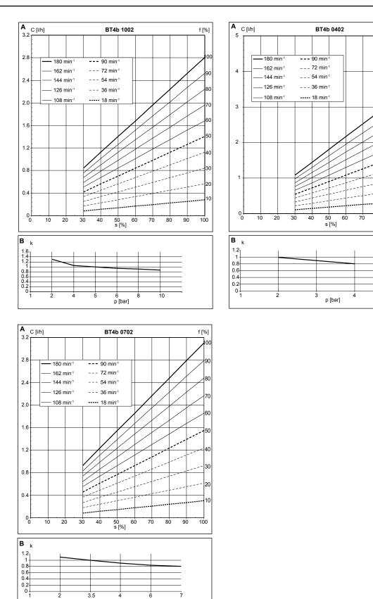
*Fig. 28: A) Capacity C at medium back pressure depending on the stroke length s for different stroke rates f. B) Associated correction factors k depending on the back pressure p.*
