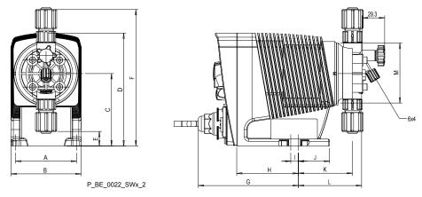
Fig. 22: Dimension drawing Beta b BT4b/BT5b, material version PV - dimensions in mm
