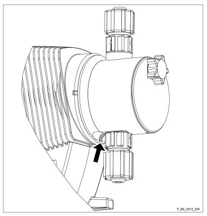
Fig. 17: The leakage hole
