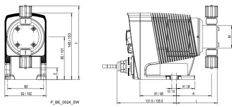
Fig. 24: Dimensional drawing Beta b BT4b/BT5b, material version TT - dimensions in mm
