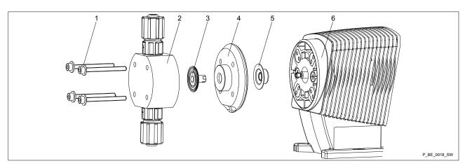
Fig. 18: Partially exploded view of the liquid end
