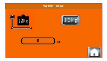
2. Once the electronics has recognized the zero weight, the certified weight of 10 kg that accompanies the equipment will be carefully deposited on the platform of the scale.
