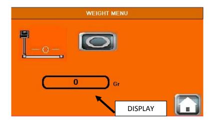
1. Firstly, it will be verified that there is no object, liquid or weight on the platform of the scale and will proceed to press the button so that the control electronics accept the current weight as weight in empty. The system will take a few seconds to acknowledge it. At that moment, the value 0 will appear in the display.
