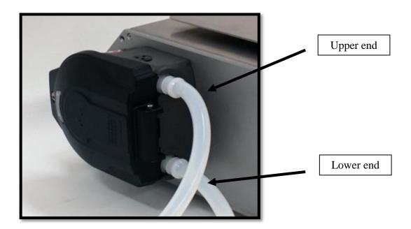
Connect the upper end of the hose to a 100-cm-long silicone tube and extend the tube through the support mast to the clamp, as shown in the image below. Bend the tube correctly over the clamp to guarantee accuracy. A tube bent in excess or defect may affect dosing accuracy. You should adjust the length of the curve to the length of the clamp, as in the picture below:
