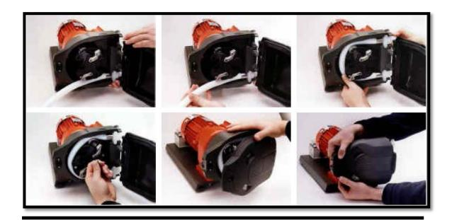
The procedure for inserting the hose is similar. Once placed the hose, make sure the two plastic ends fit in the slots of the headpiece and spread the steel rollers using the lever, enabling the pumping.
