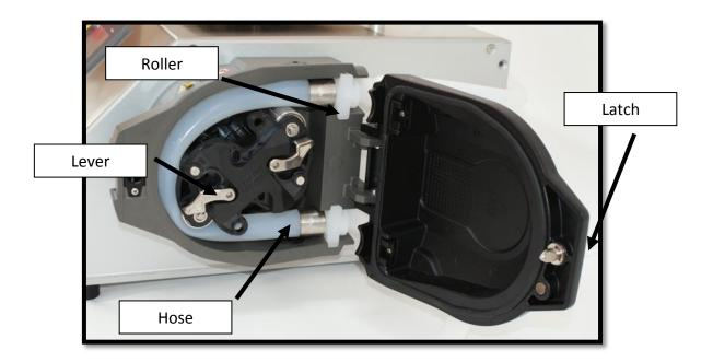
The peristaltic pump uses a removable silicone hose (included) to pump the fluid in the best sanitary conditions. Such piece can be extracted and cleaned (it is recommended to clean the hose before running the machine for the first time).
