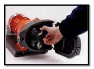
It is advisable to replace the hose yearly or every 50,000 liters pumped. The useful life of the hose depends on the run speed selected (nominal or quick), the cleaning method applied (alcohol, heat, autoclave) and the maintenance of the impeller (lubrication). If autoclave is applied, the hose only admits 3 cleaning cycles. The ends of the hose can be attached to a standard silicone piece of 16 mm of diameter by simple manual strapping:
