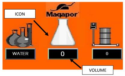
Enter the value of the volume to be measured in milliliters (eg 2500 ml) as pressing on the display itself a numeric keypad will appear. Then press F1 (RUN) for a couple of seconds. After them the machine will start the pump until the requested volume is dosed inside the container. A bar graphic will show the percentage of dosed fluid in relation to the total.
