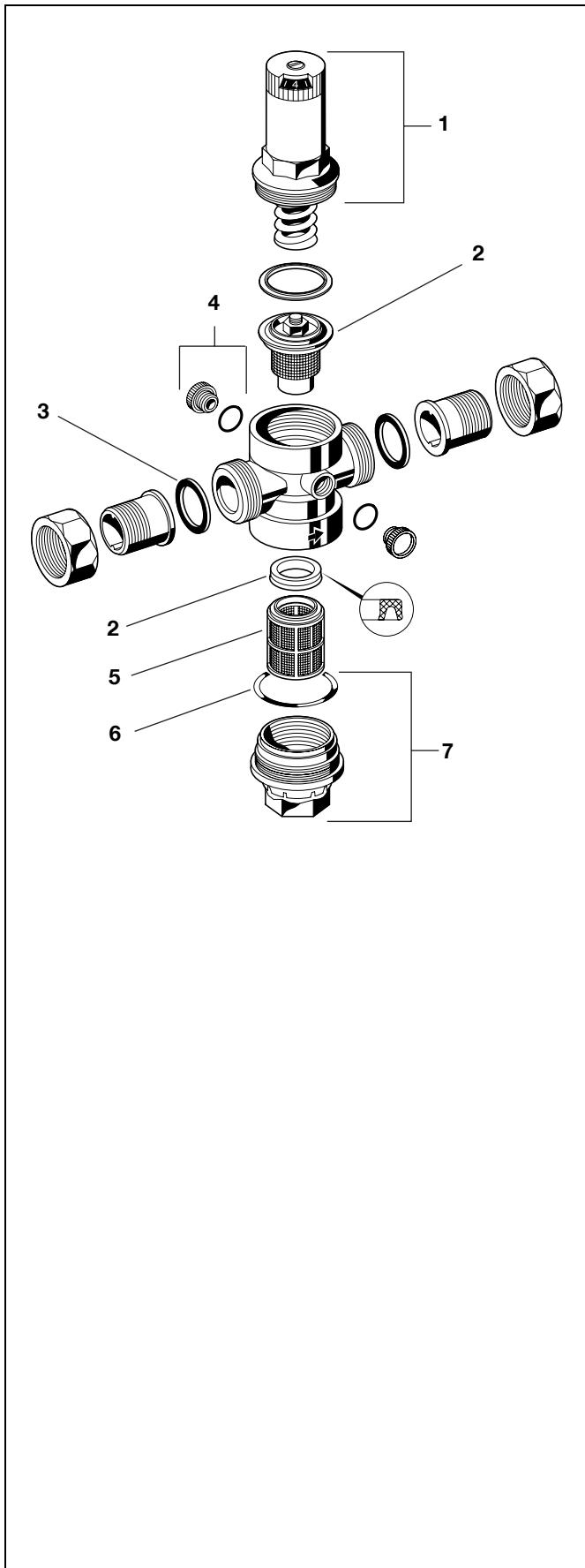
**Spare Parts****Pressure Reducing Valve D06FI, from 2007 onwards**
