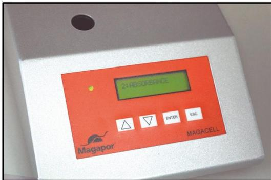
Use this option to work with absorbance, i.e., directly reading the absorbance of a sample and working with it afterwards.
