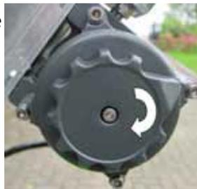
Turning the winch to the freewheel position
