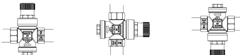
7. The final adjustment of the pressure reducing valve has to be carried out with a filled private water system and with all the outlets shut-off. The upstream pressure has to be at least 1 bar higher than the adjusted pressure.
