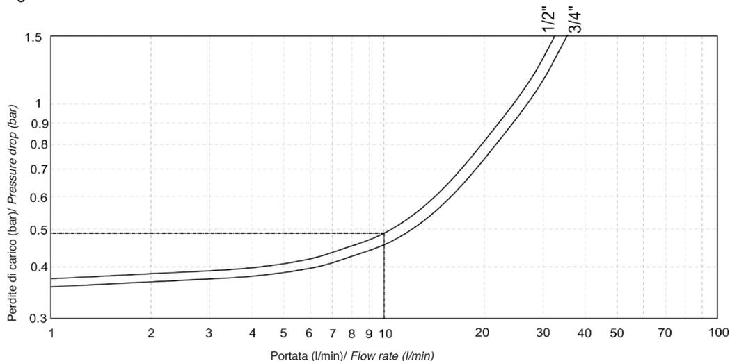
Here mentioned figures refer to: upstream pressure 8 bar downstream pressure 3 bar
