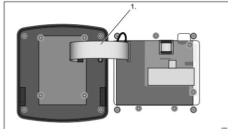
Fig. 49: Loosen the ribbon cable from the base
