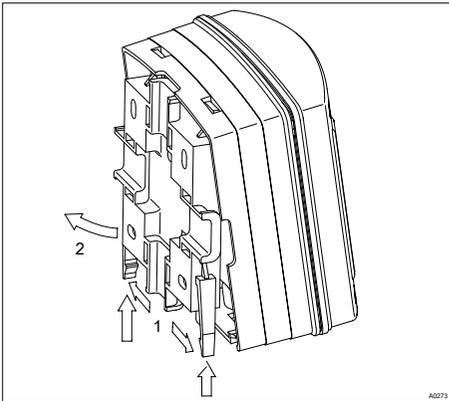
Fig. 5: Removing the wall/pipe bracket
