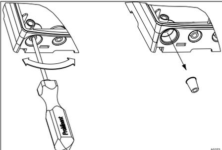
Fig. 46: Punching out the threaded holes
