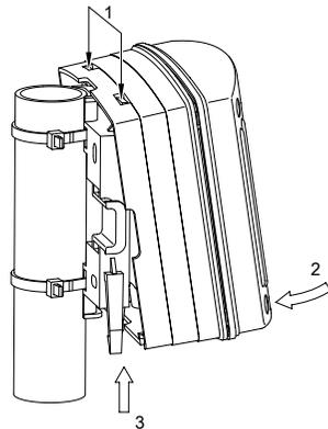
Fig. 6: Suspend and secure the DULCOMETER® Compact Controller
