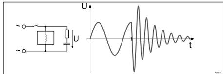
*Fig. 17: Switching-off process shown on the oscillogram.*
