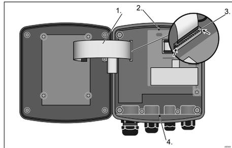
Fig. 44: Loosening the ribbon cable
