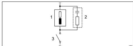
*Fig. 18: RC protective circuit for the relay contacts*
