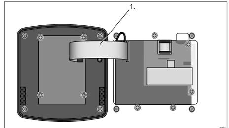
Fig. 42: Pushing and locking the ribbon cable in its base
