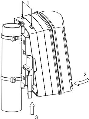
Fig. 48: Suspend and secure the DULCOMETER® Compact Controller
