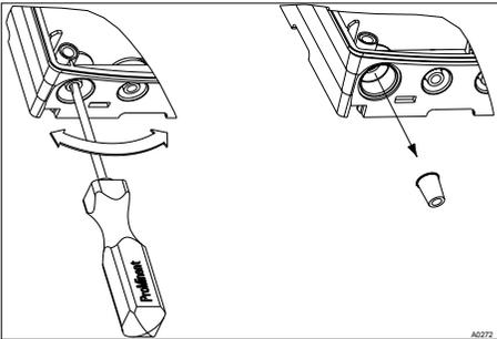
*Fig. 16: Punch out threaded holes*
