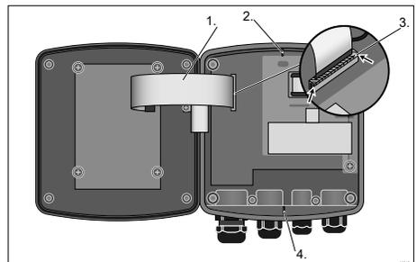
Fig. 47: Fix the ribbon cable
