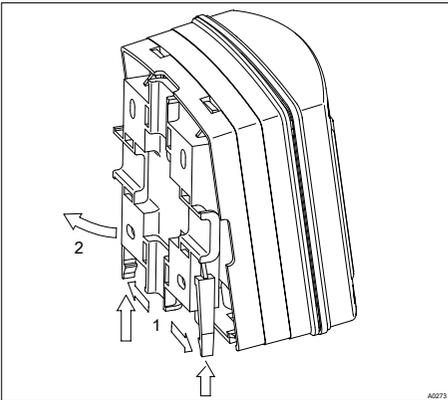
Fig. 43: Removing the wall/tube retaining bracket
