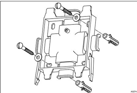
Fig. 4: Screwing on the wall/pipe bracket using washers
