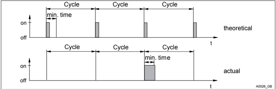
Fig. 37: Theoretical switching time < min. time
