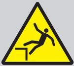
Warning of danger of falling when using fold-out steps
