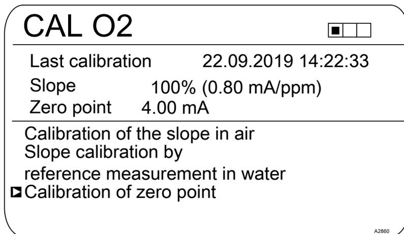
Fig. 56: Introduction: Calibration of the zero point
