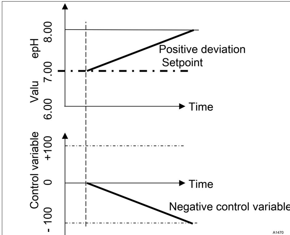
Fig. 64: PID monidirectional control type, pH-lowering
