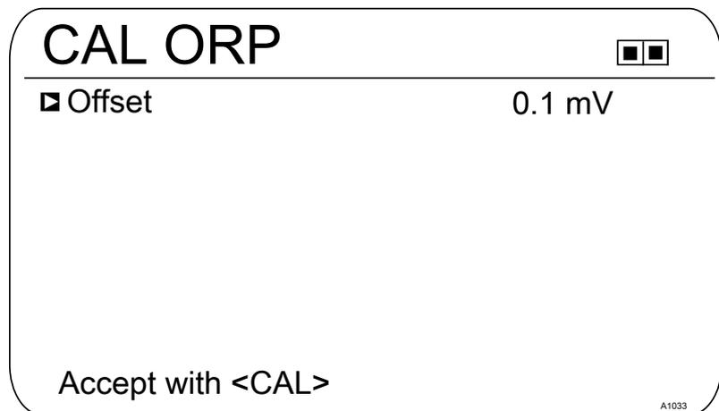
Fig. 32: Adjusting the [Offset]
