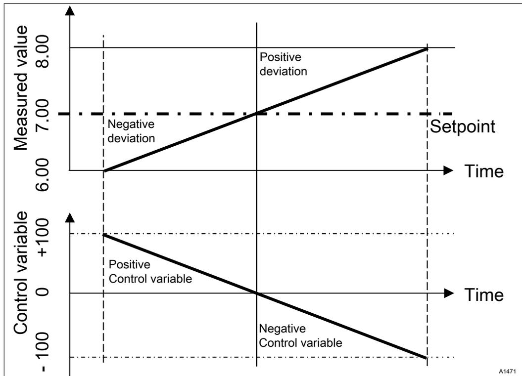
Fig. 62: PID bidirectional control type. Control characteristic without dead zone
