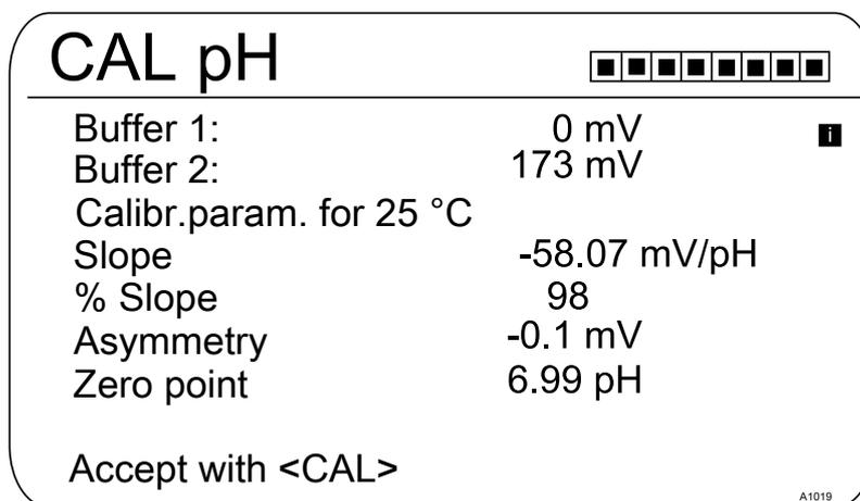
Fig. 21: Display of the calibration result
