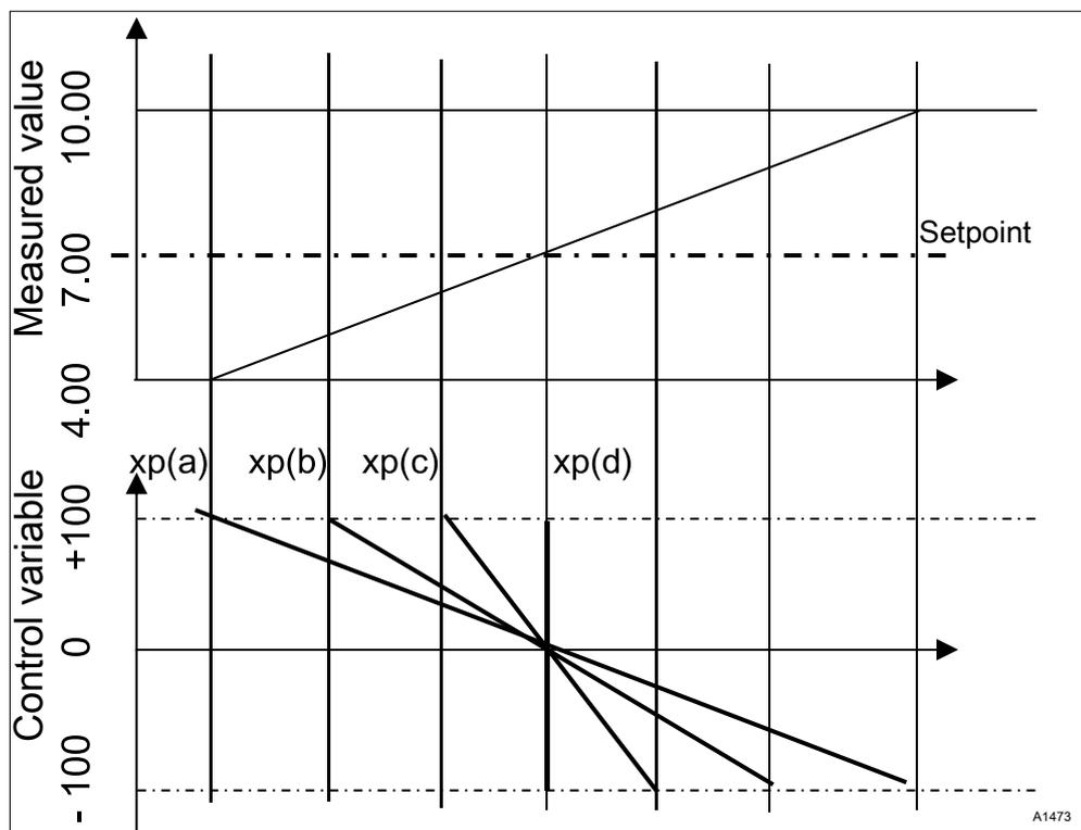
Fig. 66: The smaller the xp value, the more "forcefully" the control reacts.
