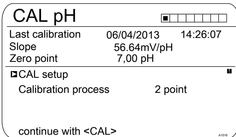
Fig. 18: pH sensor calibration (CAL)
