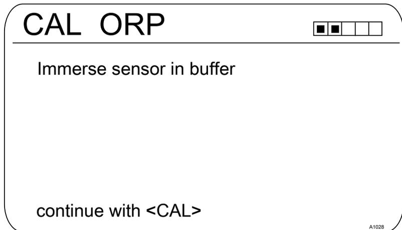
Fig. 28: 1-point calibration of ORP sensor (CAL)
