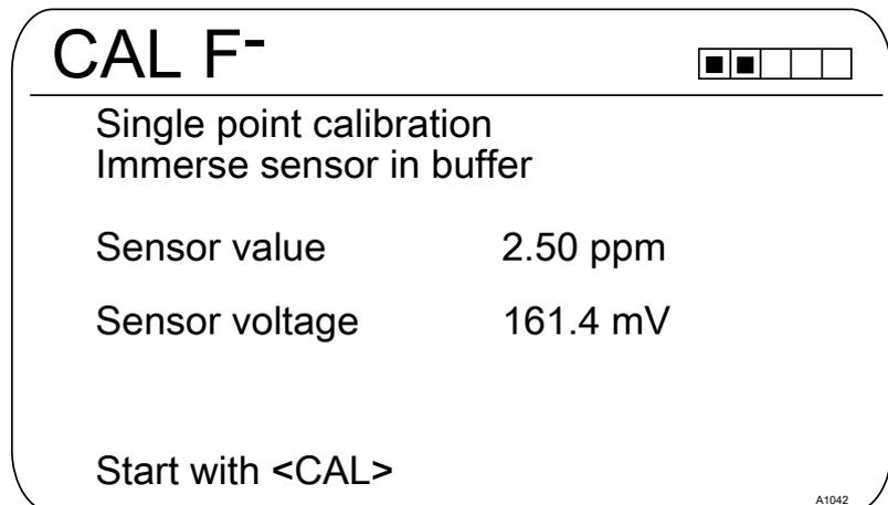
Fig. 37: Fluoride sensor calibration (CAL)
