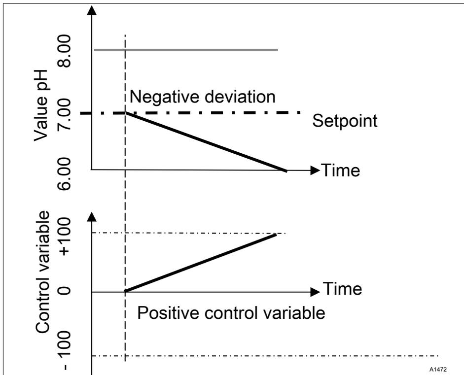
Fig. 65: PID monidirectional control type, pH-raising
