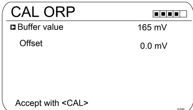
Fig. 30: Adjusting the buffer value
