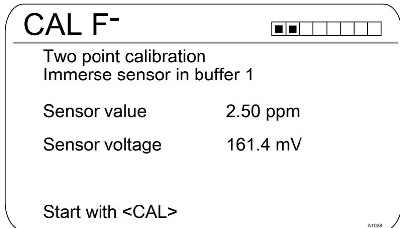
Fig. 34: Fluoride sensor calibration (CAL)
