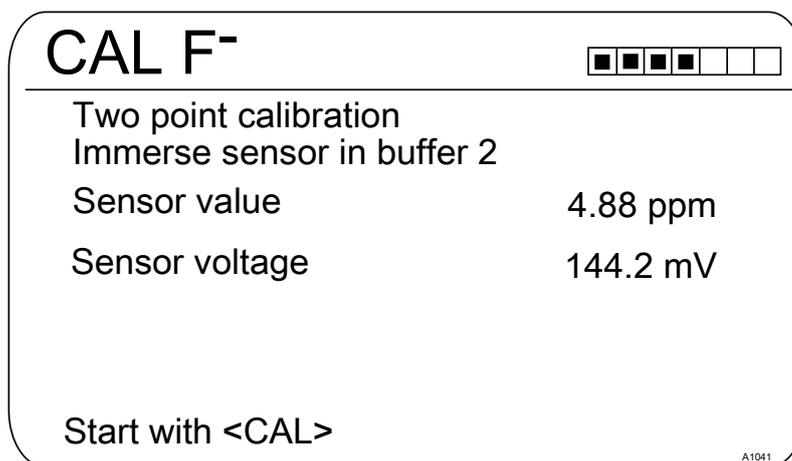
Fig. 36: Fluoride sensor calibration (CAL)
