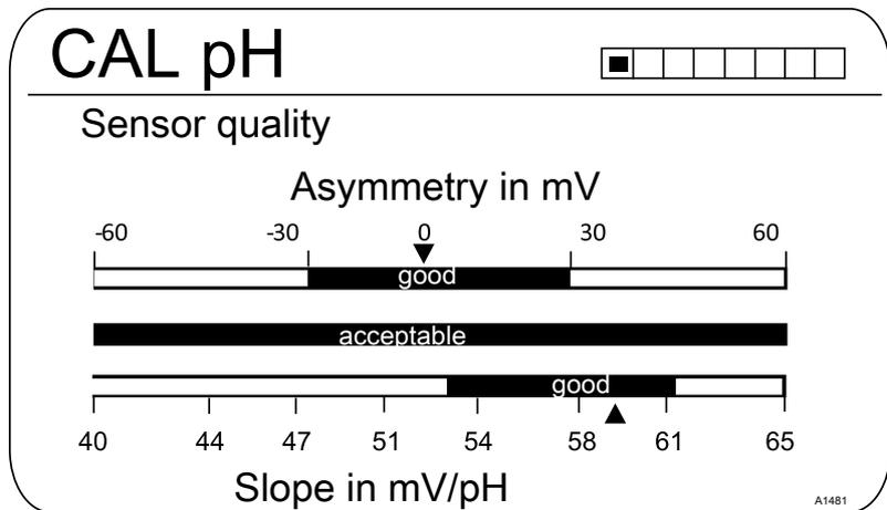
Fig. 15: Displayed after the ► key has been pressed
