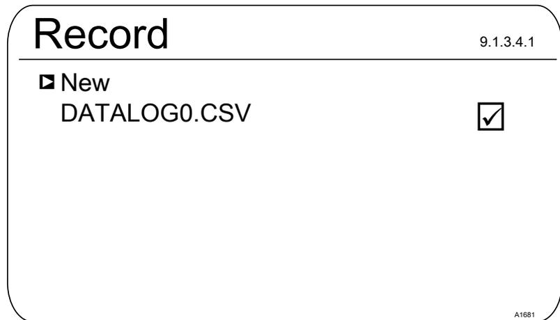
*Fig. 97: Check the file to write it to an existing file, here [DATALOG0.CSV]*
