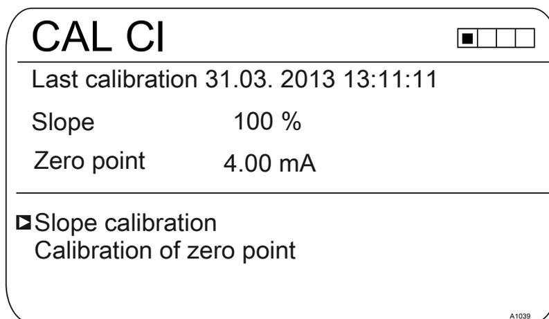
Fig. 13: [Calibration] display using [Chlorine] as an example.
