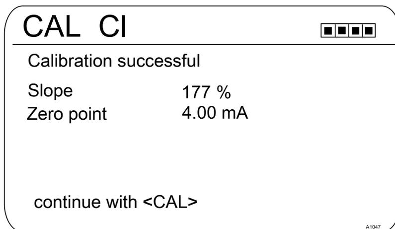
Fig. 42: Calibrating the reference value
