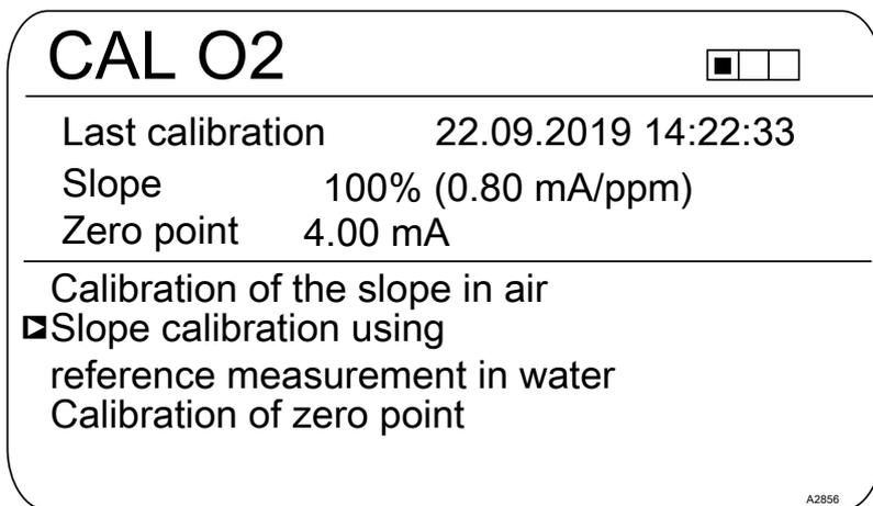
Fig. 50: Calibrating the slope using a reference measurement in water
