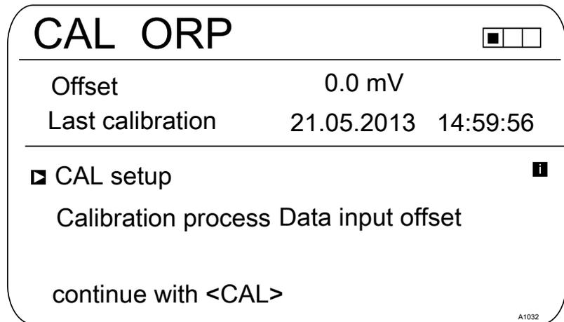
Fig. 31: Data input, ORP sensor calibration (CAL)
