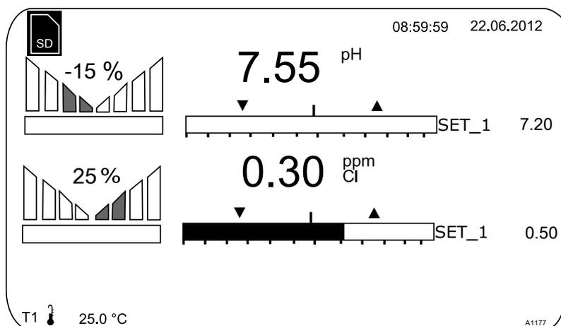
Fig. 87: Display showing symbol for the presence of an SD card (top right)
