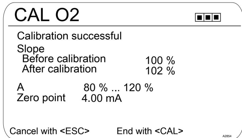
Fig. 48: Successful calibration
