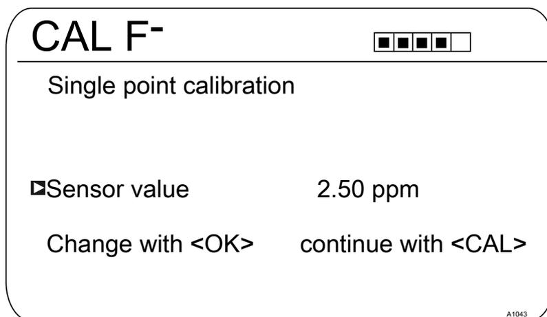
Fig. 38: Fluoride sensor calibration (CAL)
