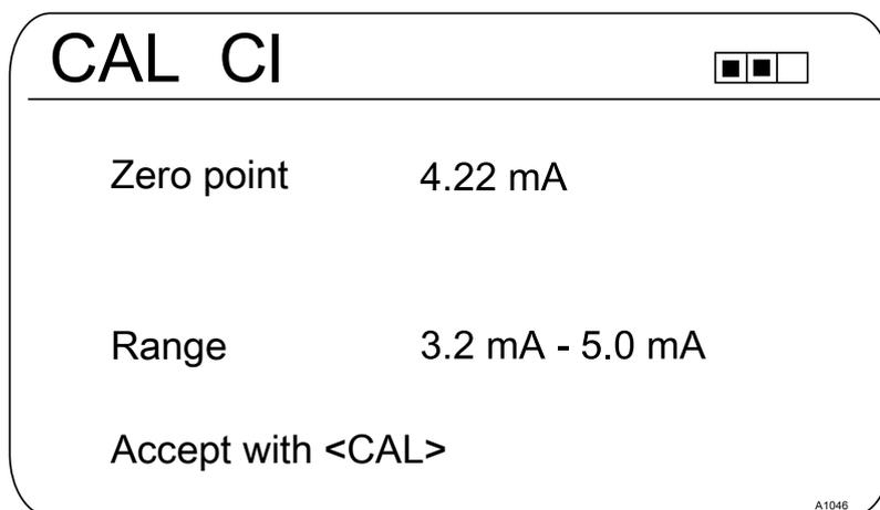
Fig. 43: Calibration of zero point
