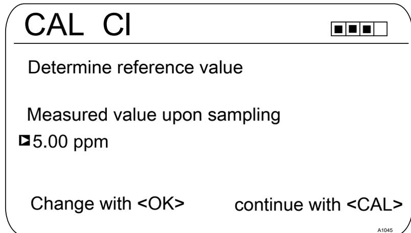
Fig. 41: Reference value calibration, the sensor value is frozen here; now take the sample and measure using DPD, for example
