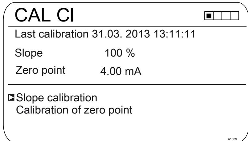
Fig. 39: [Chlorine] calibration menu
