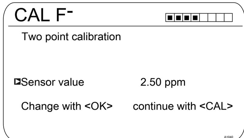
Fig. 35: Fluoride sensor calibration (CAL)
