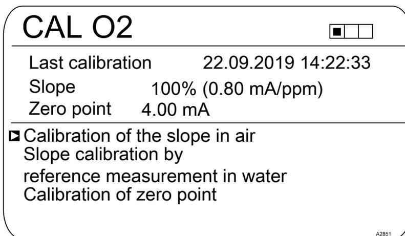
Fig. 45: Calibration of the slope in air
