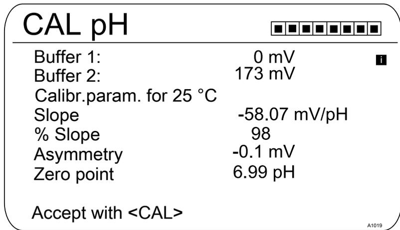
Fig. 14: Display of the calibration result
