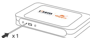
T-Sem can also perform the synchronisation cycle in manual mode, by pressing its button once.
