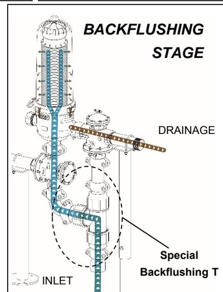
The end of the backflushing coincides with the closure of the drainage outlet and the opening of the outlet manifold, allowing water coming from the feeder manifold to come into the interior of the filter and in this way, to re-establish the filtration phase conditions.
