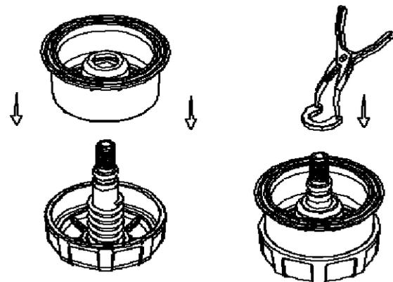
**3.** Place the piston in the filtering element, lubricate the base of the filtering element with a product chemically compatible with the material of the filter and introduce the filtering element pushing it carefully in the base of the filter. (see sections **Cleaning of discs**).
