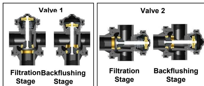
The available hydraulic power is used to overcome the pressure exerted by the spring on the discs stack generating in this way its own decompression due to the piston displacement (raising).
