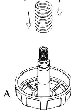
**3.3.** Introduce the B Piece on the axis of A piece. Fit the ring on the axis of B piece using the pliers until it fix in the groove of the rod.
