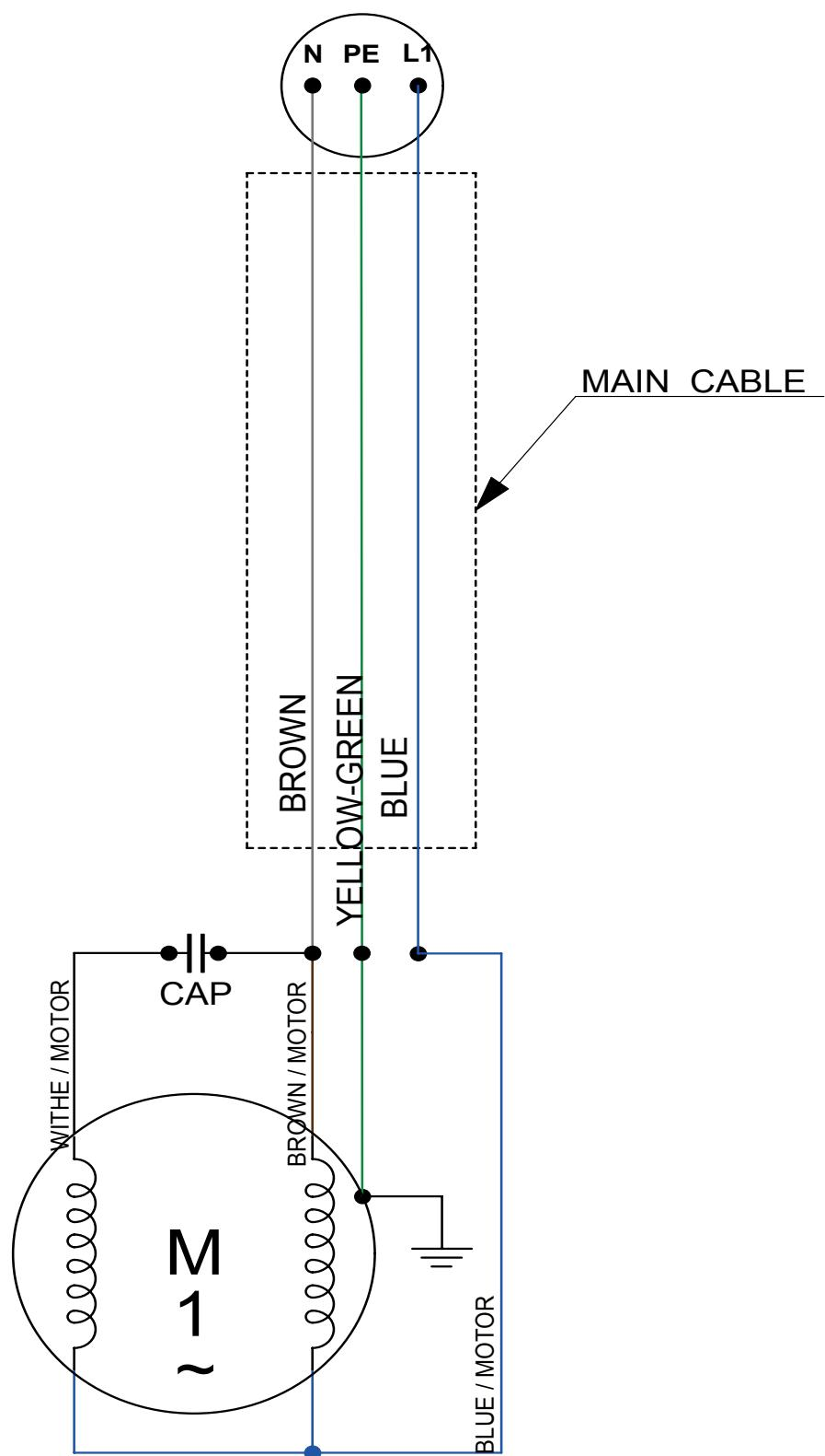
2. Electric pump 1~ with floating switch
