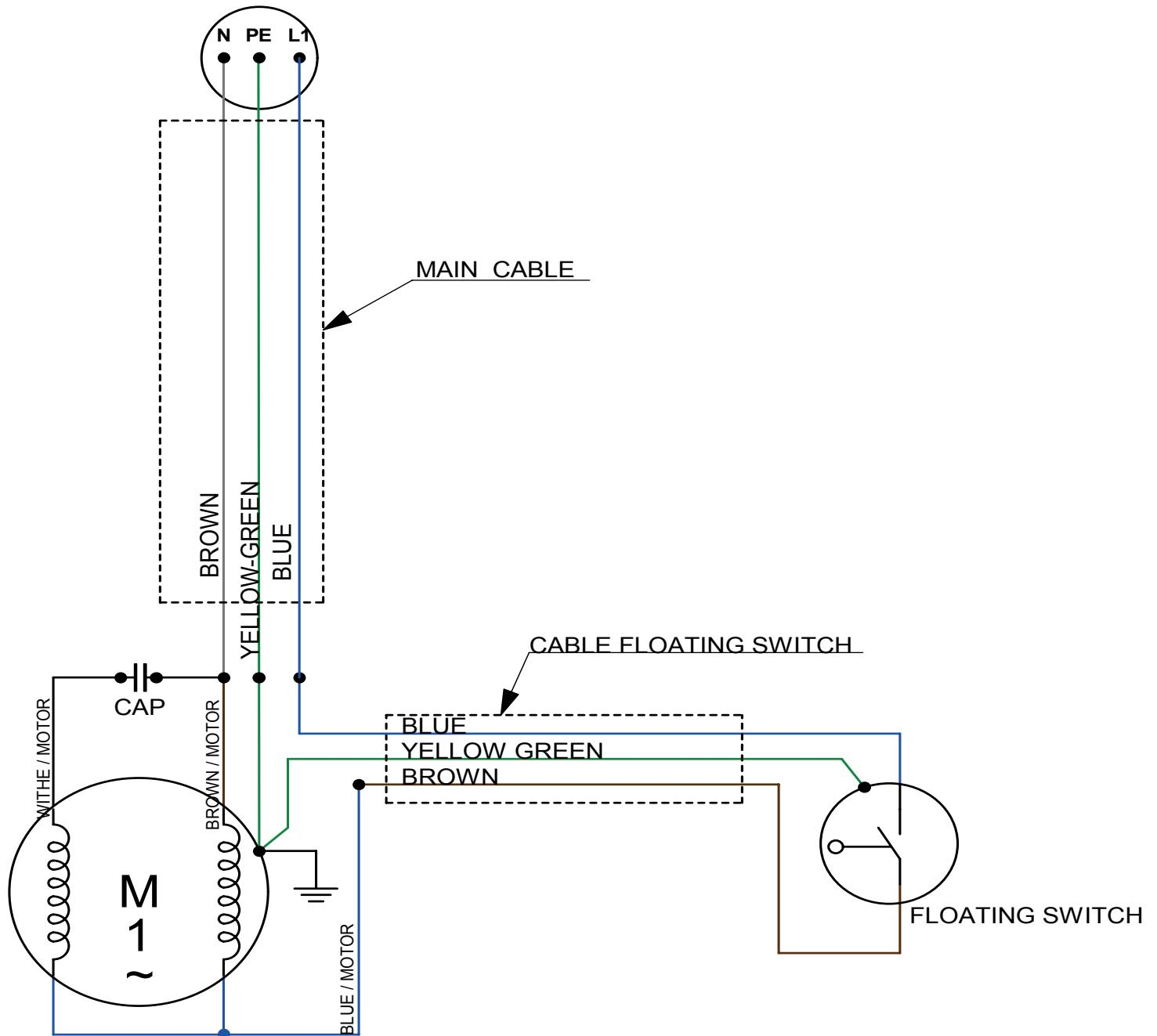
1. Electric pump 1~ with floating switch and control box
