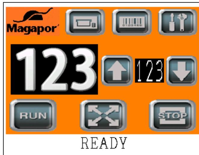
This menu contains the start and stop buttons of the machine and gives access to additional menus for setting up parameters or entering information.
