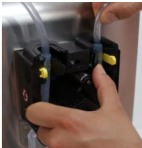
See the result in the previous picture. To end with, close the cover of the peristaltic pump by pressing. Note the pump always turns clockwise during the run, except when the manual reverse is activated for the emptying of the tube.
