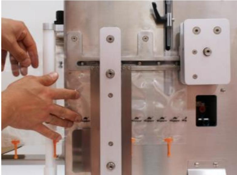
Pull the blisters manually till the opening of the first bag stands just below the filling needle or punch and the upper holes of the blisters match the poles (cylinders) of the horizontal guide.
