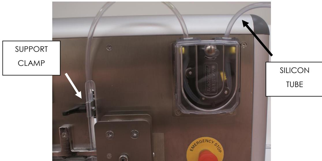
The needle will be inserted in the support clamp, loosening the locking butterfly screw. Do not tighten it again yet, because it will be necessary to make another operation after calibrating the peristaltic pump which involves removing the needle from the clamp.
